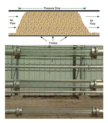
Material travels at significantly reduced velocity
