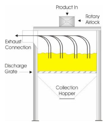
Figure 2. Typical vertical cooler arrangement.
