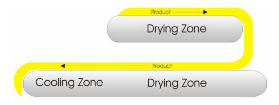
Figure1: Illustration of a combination horizontal dryer/cooler.
