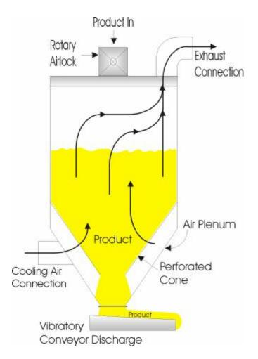
Figure 4. Illustration of a vertical cooler manufactured by Extru-Tech, Inc.
