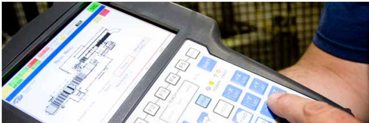
Color teach pendant used as main interface on standard palletizing cell
