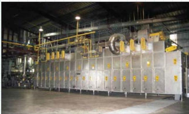
ple-pass petfood conveyor dryer, and the first sequentially-zoned dryer to optimize control of each phase of drying using independently-controlled zones.
