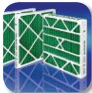
DP and DP Max pleated filters feature a proprietary high-loft media that is exclusive to Airguard. This uncharged media is a special blend of cotton and polyester fibers whose dust-holding capacity increases as the filter loads. The 4-inch deep pleats have individual die cut fingers that separate and stabilize each pleat for maximum dust-holding performance and longer service life. Consistent pleat shape, count and spacing assure best-possible performance.
