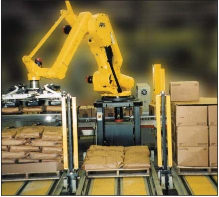
A robotic system simultaneously palletizes two bag production lines and one box production line.
