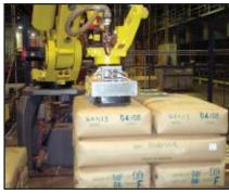
This system palletizes (or depalletizes) 100-lb. jumbo bags from two production lines simultaneously.
