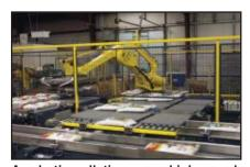
A robotic palletizer uses high-speed, full-layer forming techniques to arrange 20-50-lb. bags into full-layer patterns. The infeeds automatically change over via a touch screen.
