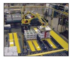
Above, a robotic palletizer is handling two bag production lines and one bundle production line.
