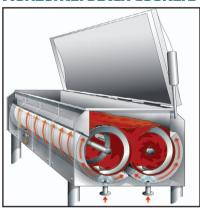
Mepaco has developed its new line of ThermaBlend cookers for viscous food products. ThermaBlend cookers have an hourglass design that provides a larger heating surface for better heat transfer, according to the company. The cookers feature dual-ribbon agitators, a wrap-around ASME heat jacket and a scraper system to prevent burnon, while maximizing even transfer of heat to the product.
