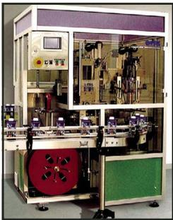
PDC International has introduced a heavy-duty, highly flexible shrink sleeving machine that runs both tamper-evident neckbands and shrink-sleeve
