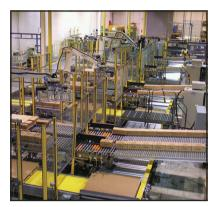
line, Columbia can provide complete turnkey solutions that incorporate conveyors, bar-code readers, case and bag elevators, bag weighers, bag flatteners, shuttle cars, stretch wrappers and more. Complete systems integration includes project management, controls, installation, wiring, commissioning and preventive maintenance from one source.
