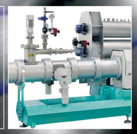
ECOtwin, the twin-screw extruder with the new SME- and Density-Control modules for independent and online control of the cooking degree and the specific weight of the product. All for your benefit!
