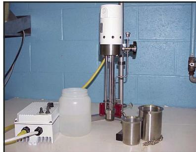
15,000 RPM reversible motor. The unique down-mode is capable of drawing and wetting out floating powders. The down-mode can also be utilized to re-suspend any settled solids on the bottom of the process mixing vessel. The mixer comes complete with a stand and reversible variable-speed control box.
