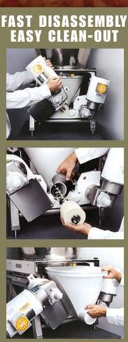
Our sanitary-grade DEA open frame weighbelt offers easy wash-down, all stainless steel construction in 12" and 24" wide belt sizes.
