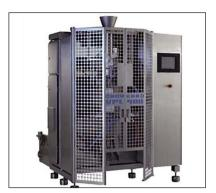
ment incorporating modern linear servo drive technology. The VPL-400 is now available for the production of flat-bottom bags and Stabilo Seal bags. The VPL-400 allows users to set functions such as sealing time, sealing pressure, cooling time, speed and all jaw movements, both vertical and horizontal, for highest performance, flexibility and top seal quality, according to Rovema.
