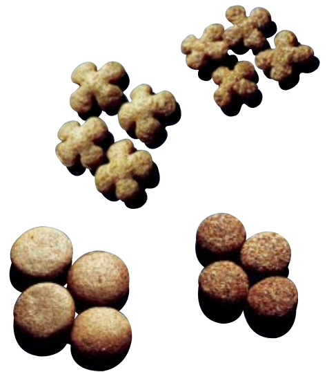
The particle size and pre-grinding of raw materials is especially critical if the final product is a delicate shape. The samples on the left were ground through a 0.8 mm hammermill screen, the ones on the right through a 1.5 mm hammermill screen.
