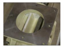
ner diameter of the housing and the end plates. Airlocks can be rebuilt to specified tolerances, using either carbide or ceramic tiles depending on customer requirements. Machining and grinding capabilities allow modification of the areas to be protected so they can accept any specified coating or lining, which can then be ground to meet exact tolerances.
