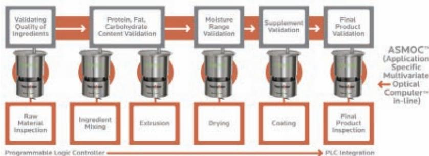
**A challenge in the petfood industry is providing high-volume process logic control for both wet and dry petfoods at multiple control points, from the introduction of ingredients to final validation.**
