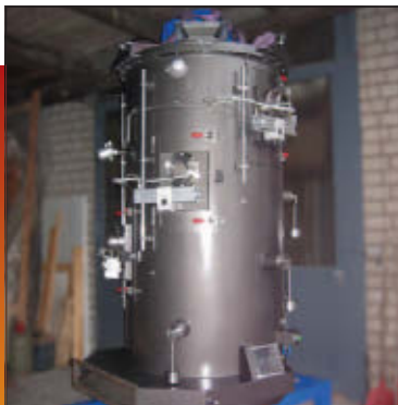
What makes Münch-Edelstahl's Carousel Dryer/Cooler different from other counterflow drying systems is the cylindrical body. The round profile of the Carousel allows gentle and uniform drying of the product.
