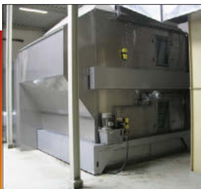
Counterflow dryers, like this example from Geelen Counterflow, already have over 50% market share in countries such as Japan, France, Spain, Italy, Belgium, the Netherlands and Argentina.
