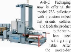
guides the layer to the pallet stack, each layer is tightened and squared by the four-sided squaring device.
