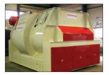
liquids can be oil-, water- or acid-based. The machine mixes quickly, making it possible to realize energy savings of 30% to 40%, according to the company.
