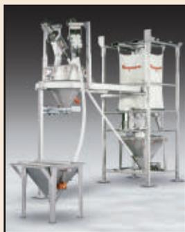
system that weighs bulk materials discharged from bulk bags or manually dumped from sacks, boxes and other containers and empties the batch into mobile-storage bins. The sanitary system consists of a bulk bag unloading frame, two hoppers and two flexible screw conveyors that feed a central gain-in-weight hopper under automated control.
