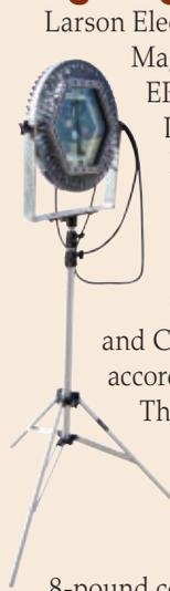
Larson Electronics LLC's Magnalight offers an EPL-BS-161M-TP1-100 LED light for hazardous locations. The tripod mounted LED light is UL rated as Class 1, Division 1, Groups C and D, and Class 2, Division 1 - 2, according to the company. The 16-inch LED light head produces 10,000 lumens of light from 150 watts, the company says. An 8-pound collapsible tripod
