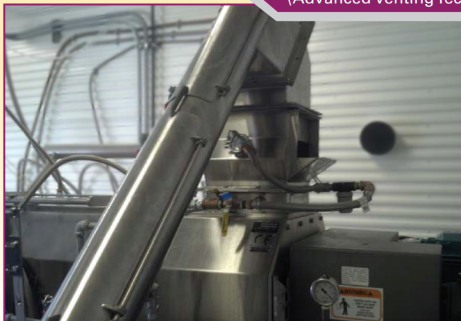
Conditioning Cylinder Inlet: Inoculation Port with AVT (Advanced Venting Technology)
