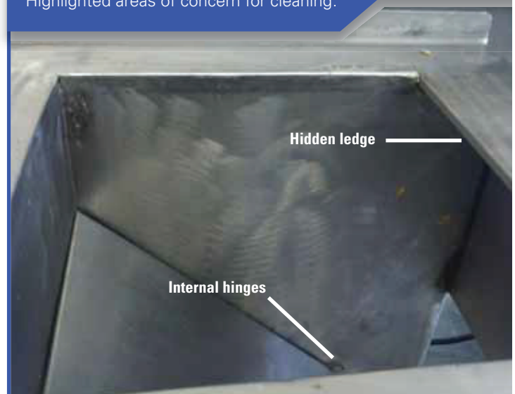
Figure 3. ADP Downspout Diverter – Highlighted areas of concern for cleaning.
