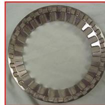
The function of the lug ring is to restrict product swirl in the cutting chamber while at the same time, provide additional cutting action in the chamber. Lug rings are available in various lug configurations and are designed to fit your needs, from stainless steel to tool steel materials.
