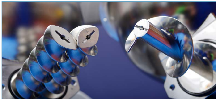
Figure 1: Twin and single screw feeders are used for a wide variety of raw materials
