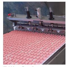
**Multi-Lane Extruding** The Vemag and a Waterwheel attachment extrude multiple lanes of pellets, meat sticks and jerky with consistent thickness, width and length.
