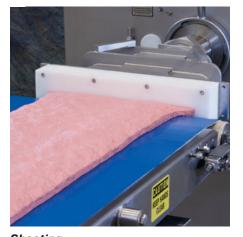
**Sheeting** The Vemag and a Sheeting attachment extrude smooth, uniform, continuous sheets of product with consistent thickness and width.
