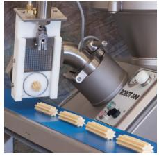
**Shape Forming & Portioning** The Vemag and various Shape Forming attachments extrude a wide range of unique shapes, bars, and meatballs – all with consistent shapes and weights.
