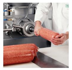
**Grinding & Portioning** The Vemag precisely grinds and portions fresh product into chub packaging and is easily adaptable for all types of products and outputs.
