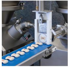
**Coextruding & Portioning** Two Vemags and a Coextruder attachment produce an endless assortment of exact-weight filled treats.
