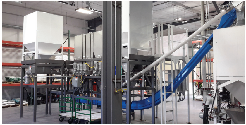
Figure 1: Twelve (12) Bin Micro Ingredient System with Four (4) Bulk Tote Bins; System Uses Three (3) Ingredient Scales and One (1) Batch Check Weigh Scale; Seven (7) 3" Auger and Five (5) 4" Auger Multiple Speed Feeders.
