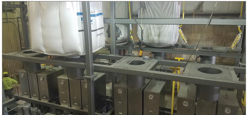
Figure 2: Twenty-Four (24) Bin Micro Ingredient System with Eight (8) Bulk Bag Bin Inlets; System Uses Four (4) Micro Scale Hoppers; Sixteen (16) 3" Auger and Eight (8) 4" Auger Multiple Speed Feeders; Weigh Cycle 2-3 Minutes (Prior to installation of micro system batch cycle time was 10-13 minutes)
