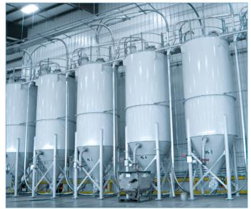
Coperion K-Tron pneumatic conveying system
