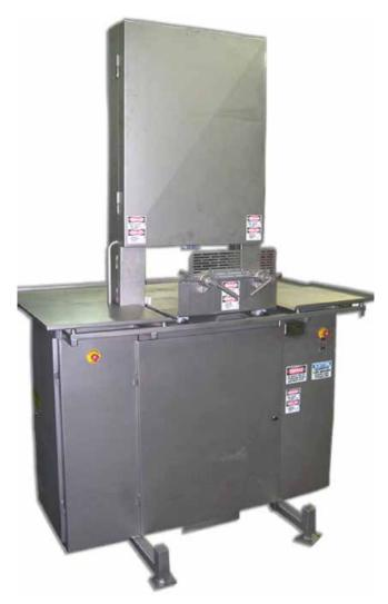
Midwest Metalcraft's Multi-Blade Saw offers a unique solution for operations needing to make several cuts of the same thickness. These types of cuts require the operator to work in close proximity to the cutting blade which can be dangerous and time consuming. The Midwest Metalcraft's Multi-Blade Saw addresses these issues and provides superior accuracy and productivity.
