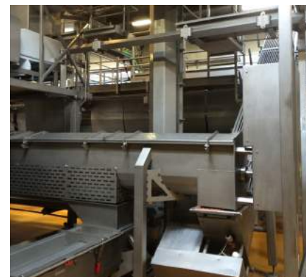
scansteel foodtech Whole Pallet Crusher, WPC 2000-Single, shown in application where existing footprint is sparse and where the pre-broken frozen blocks need to be elevated to approx. 5000 mm.
