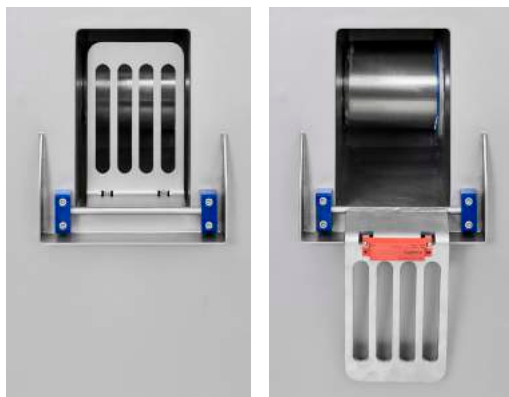
A prime example of scansteel foodtech's hygienic design is given by the hygienic zone positioned between the worm/auger and the gear box. Hygienic zone shown in running position (closed) and in cleaning/inspection position. When opened the grinder cannot be started until the guard is positioned in closed position. = When opened, the grinder cannot be started until the guard has been positioned in closed position.
