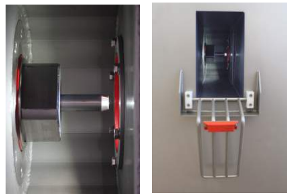
A prime example of scansteel foodtech's hygienic design is given by the two hygienic zones – one positioned between each of the worms and one between the gear boxes.
