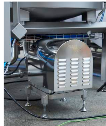
Pumps are positioned/mounted on own frame for easy access at inspection/maintenance, etc. In addition, the pump of the scanGravy mixing unit can be equipped with its own knife system for eliminating lumps in "challenging to produce" gravies.
