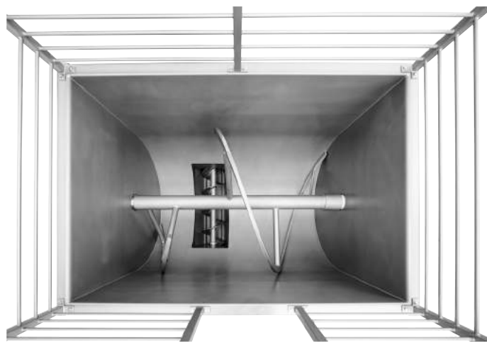
Top view of scansteel foodtech standard scanGiraff, showing stirring/feeding device.
