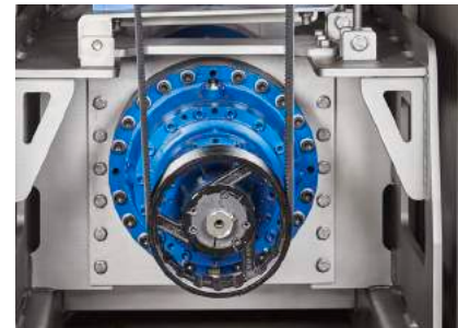
Planetary gear box assembly. Between gear box and crusher claw, a Heavy Duty safety clutch prevents damage to the gear box, example only, in case a large foreign (metal) object by mistake is thrown into the Whole Pallet Crusher.
