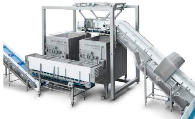
Example of inclined belt conveyor with metal detector.
