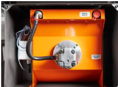
Built-in oil cooler for each gear box. Dramatically increases lifetime of the gear box securing the Whole Pallet Crusher can run 24/7 without being overloaded.
