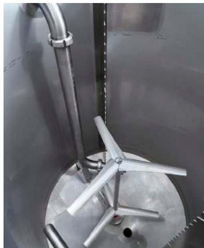
Mixing container designed for heavy viscous gravies/mixtures. The Venturi system in combination with the Heavy Duty mixing agitators ensures a fast processing of a gravy free of lumps. Anti-vortex breakers are standard in all scanGravy mixing tanks. Direct steam injection for temperature control can be added as well.
