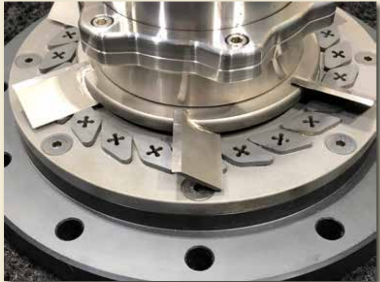
Perfectly flat, the Cutters engage the Die face with slight pressure to sharply cut product, eliminating tails and fines.
