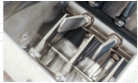
Unique counter rotating beater design lowers replacement cost and time.
