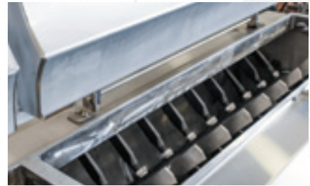
The counter weighted access doors allow quick access and are operator friendly.
