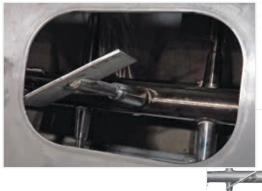
Unique rotary paddle design allows gentle material handling and reduces product degradation.
