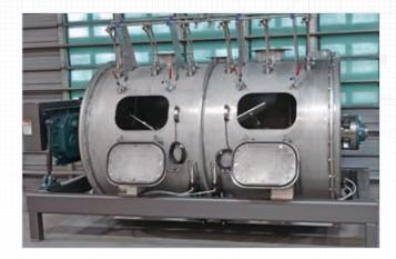
Coatings are applied in our enclosed batch mixer that features best in class product coating coverage and optimized throughput all with reduced potential for cross contamination.
