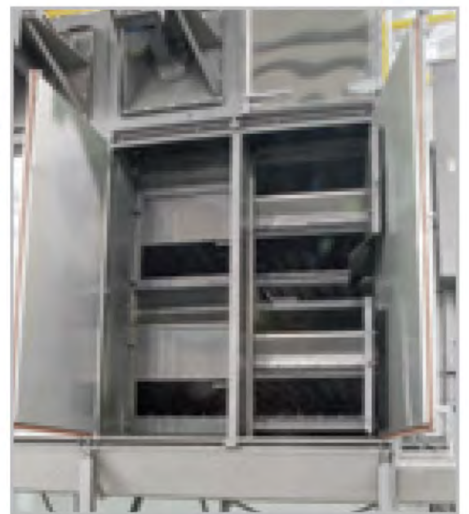
Stainless steel solid construction hinged interior doors permit easy access to product conveyors.
