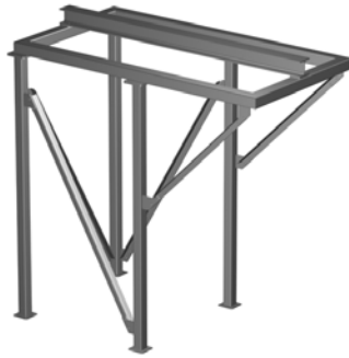
upper frame for low overall heights
