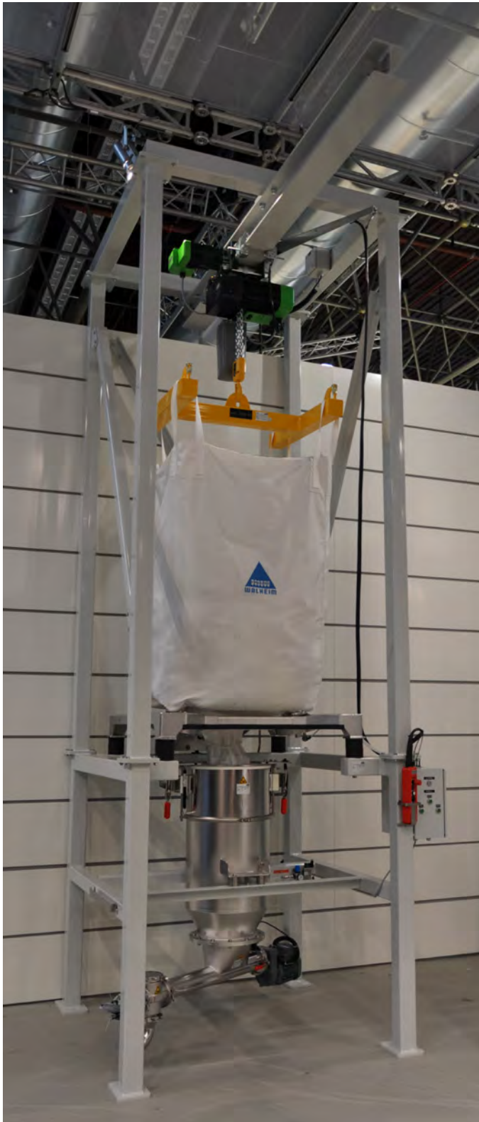
modular discharge station for big bags with mounted dosing screw (not part of the modular system)
