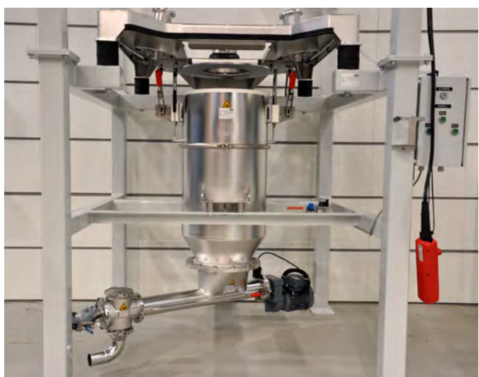
Big bag connection system with Ø 500 hopper with mounted dosing screw (not part of the modular system)
