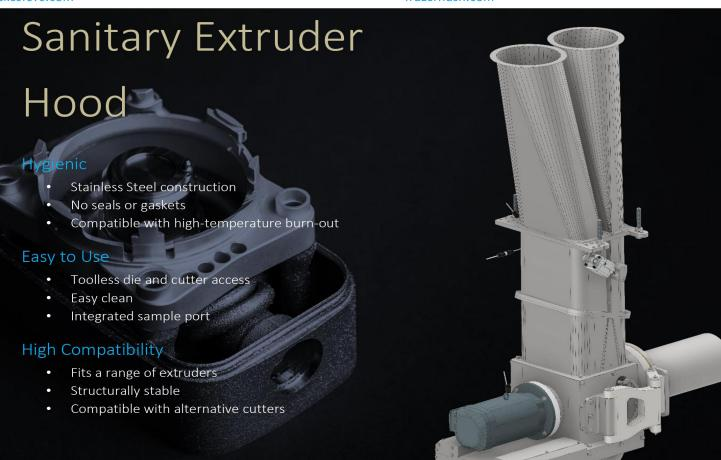
The Frazer-Nash Sanitary Extruder Hood (SEH) is used in pet food production as part of a clean air conveying system. Conditioned and filtered external air is used to prevent the risk of contamination from air within the extruder room or other parts of the factory.
