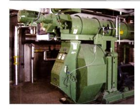
The facility was experiencing lower than desired gelatinization on its finished pelleted feed. WL Port-Land Systems worked to analyze both field data and the operation of the entire system. The analysis resulted in a need to make adjustments to the boiler pressure and steam harness pressure settings, increasing the conditioned mash moisture, resulting in improved gelatinization.
