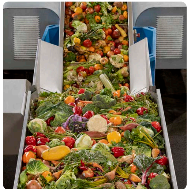
CSS Sorting line turns diverse inputs into homogenous outputs
