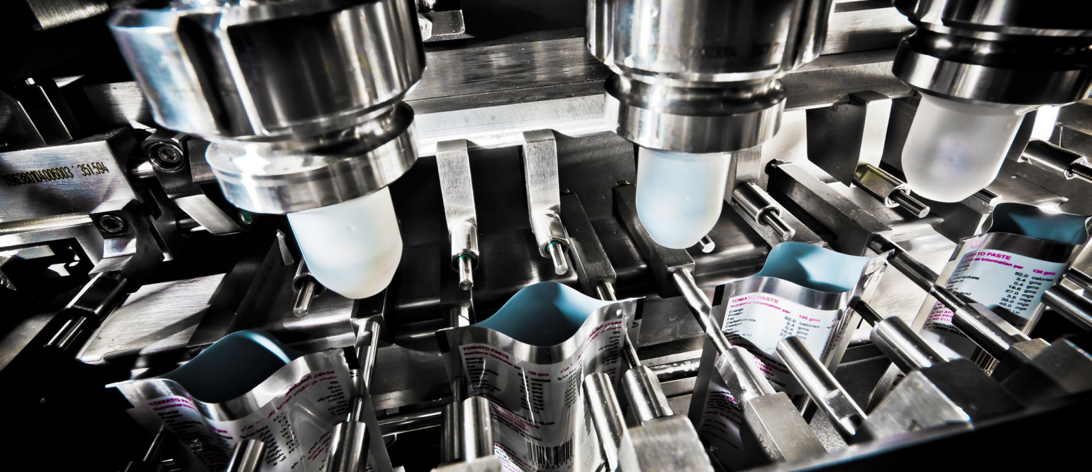
The pouch filling stage requires extreme dosing precision
