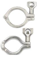
The most common type of tri-clamp is a <u>Single Pin Sanitary Hinge Clamp</u> which has a single pin on one side with a single bolt used to tighten on the other side. The fastener bolt may be a wingnut or a wing nut with a hole. In sanitary processing, these clamps range in size from ½" up to 12" and may be either 304 or 316L stainless steel.
