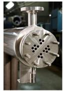
Shell and tube heat exchangers are comprised of multiple tubes through which liquid flows. The tubes are divided into two sets: the first set contains the liquid to be heated or cooled. The second set contains the liquid responsible for triggering the heat exchange, and either removes heat from the first set of tubes by absorbing and transmitting heat away—in essence, cooling the liquid—or warms the set by transmitting its own heat to the liquid inside.
