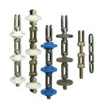
Hapman engineers will select the correct chain and flight design combination to meet your specific process and material requirements. Hapman offers link and pin type chains, which are less prone to fatigue and wear, and stretch less than steel cables. Also available are Hapman's exclusive rivetless and seal-pin chain options to fit a wider array of applications.
