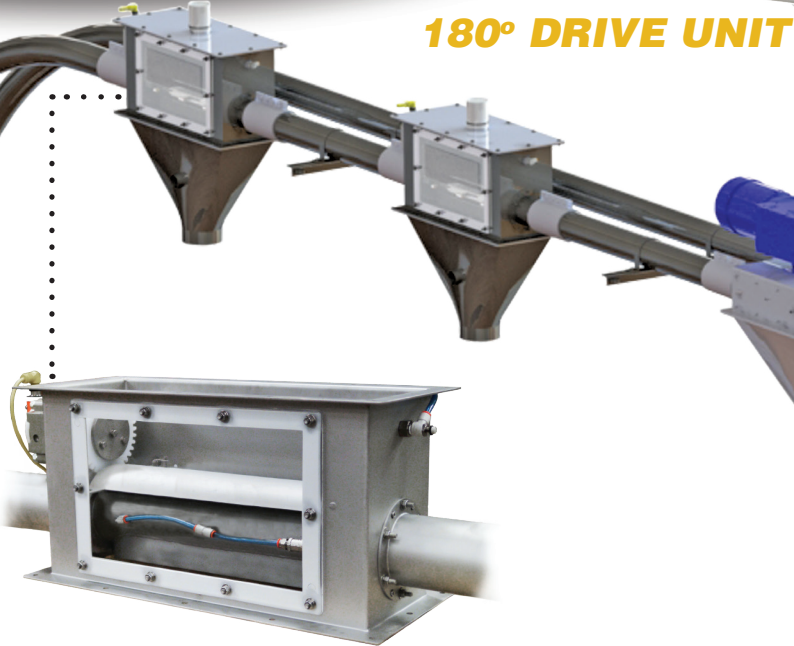
ROTARY DISCHARGE VALVE Pneumatically actuated rotary valve allows for unobstructed product discharge
