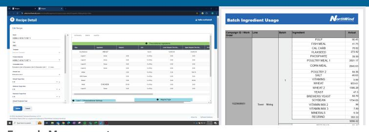
**Formula Management -** A formula consists of a list of ingredients, ingredient amounts and sequence for combining those ingredients, and the amount to be made (batch size). BatchLOGIX is a dynamic, robust program that manages the ingredients and equipment set points in both batch and continuous processes.
